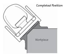
While this set-up is best for chamfering with the grain, the low cutting angle of the Veritas Low-Angle Block Plane also makes it possible to chamfer end grain.
